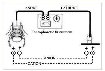
**Figure 2.** Ocular iontophoresis of a positively charged drug uses an anodic electrode to generate positively charged hydronium ions Reprinted with permission from Rajendra VB, Dhamecha DL, Deshpande ST, et al. Ocular iontophoresis: a review. *Inventi Impact.* 2011;1(3):133-136.
